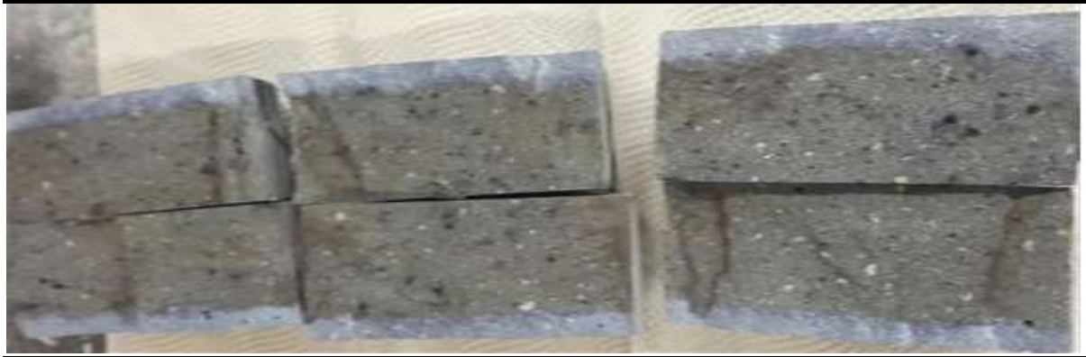
Figure 7: Chloride penetration depths of mix (a) Control mix, (b) OPC/TW30-3 and (c) OPC/TW50-3
