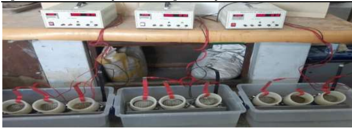
Figure 5: Pictorial view of specimens during chloride penetration test
