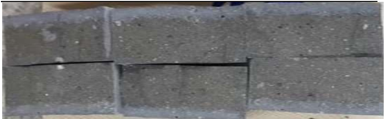
Figure 8: Chloride penetration depths of mix (a) OPC/P30-3, (b) OPC/P50-3 and (c) OPC/SAP-3
